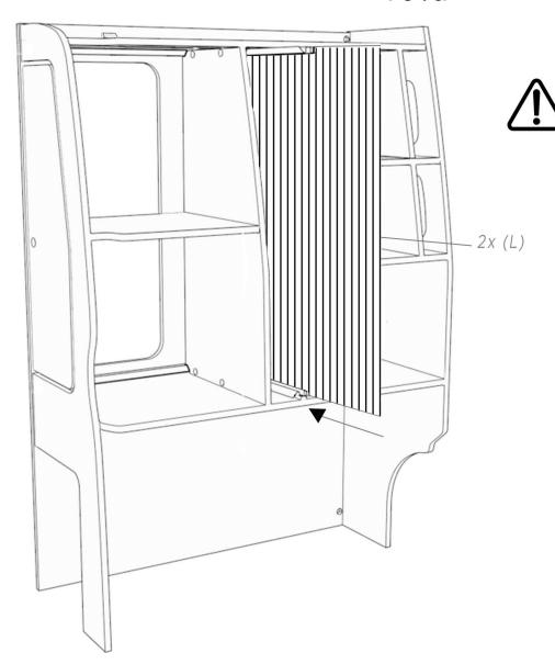
Tambour doors must be fitted BEFORE installing the wardrobe into the van.
